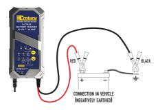
If Negatively Earthed (Most Common) – FIRST Connect the Red (+) Crocodile clip or ring terminal lead to the (+) battery terminal and then connect the Black (-) Crocodile clip or ring terminal lead to the vehicle's chassis. DO NOT connect the Black (-) lead to the carburettor or fuel lines.
