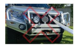
After you have attached the recovery strap to the recovery point. To reduce any injuries or damage place a dampening item over the center of the strap. This can be a tire tread or weighted bag as examples.
