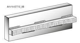
Figure 7-28: Staggered Intermittent Welding
