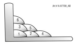
Figure 7-15: Multi-runs in HV Fillet Weld
