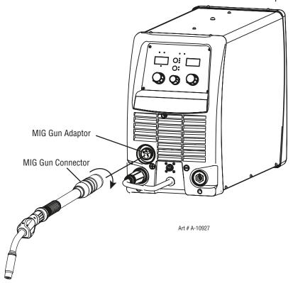
Figure 5-3: Attaching MIG Torch
