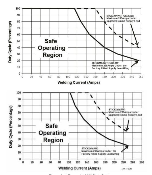
Figure 2-1: Transmig 255i Duty Cycle
