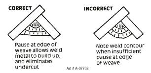
Figure 7-18: Examples of Vertical Fillet Welds
