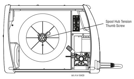
Figure 5-10: Wire Reel Brake
