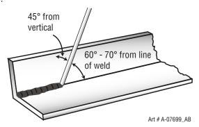
Figure 7-14: Electrode Position for HV Fillet Weld
