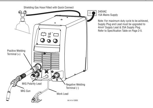
Figure 5-11: Setup for MIG Welding with Gas Shielded Mig Wire
