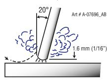
Figure 7-11: Striking an Arc
