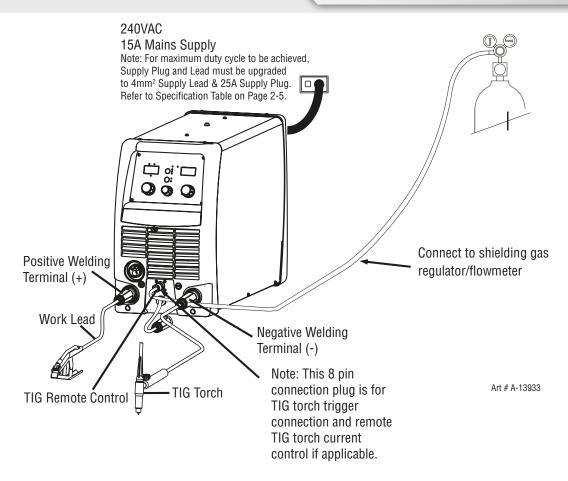
Figure 6-3: Setup for Lift TIG (GTAW) Welding
