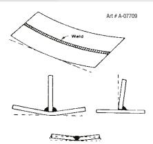
Figure 7-24: Examples of Distortion
