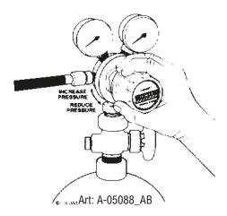
Figure 6-2: Adjust Flow Rate
