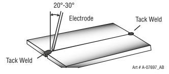
Figure 7-12: Butt Weld
