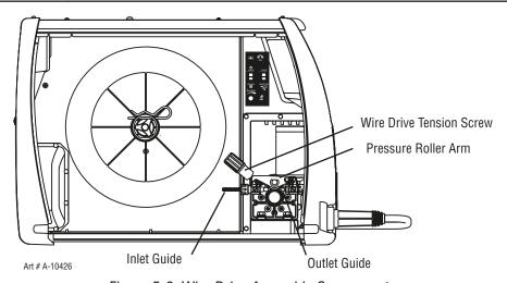
Figure 5-6: Wire Drive Assembly Components
