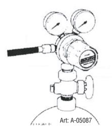
Figure 6-1: Fit Regulator to Cylinder
