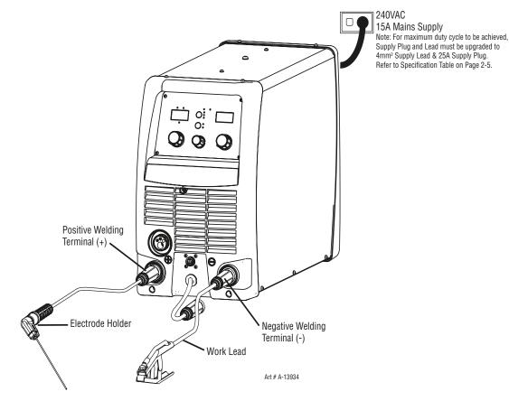
Figure 7-1: Setup for Manual Arc Welding
