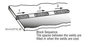
Figure 7-25: Welding Sequence
