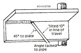
Figure 7-19: Overhead Fillet Weld
