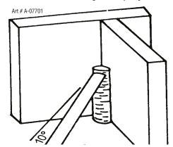
Figure 7-16: Single Run Vertical Fillet Weld
