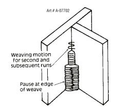
Figure 7-17: Multi Run Vertical Fillet Weld
