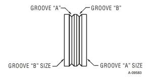
Figure 5-8: Dual Groove Feed Roller
