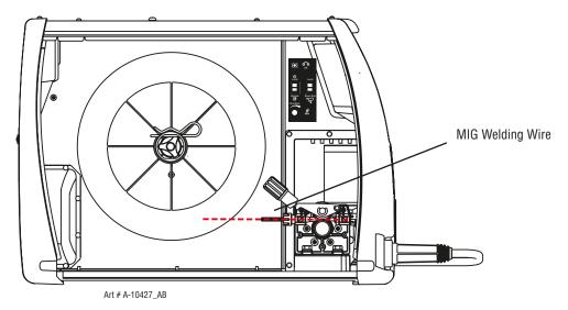
Figure 5-7: Mig Welding Wire - Installation
