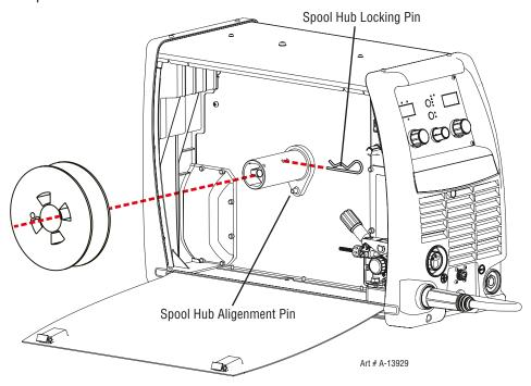
Figure 5-5: 200mm Handispool Installation
