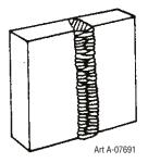
Figure 7-6: Vertical Position, Butt Weld
