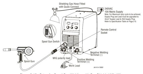
Figure 5-13: Setup for Spool Gun Welding with Gas Shielded Mig Wire
