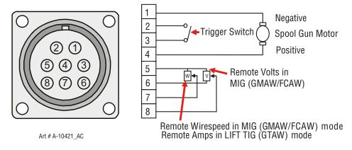
Figure 4-2: Remote Control Socket
