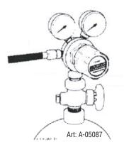
Figure 5-1: Fit Regulator/flowmeter to Cylinder
