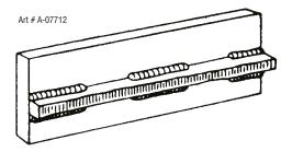
Figure 7-27: Chain Intermittent Welding
