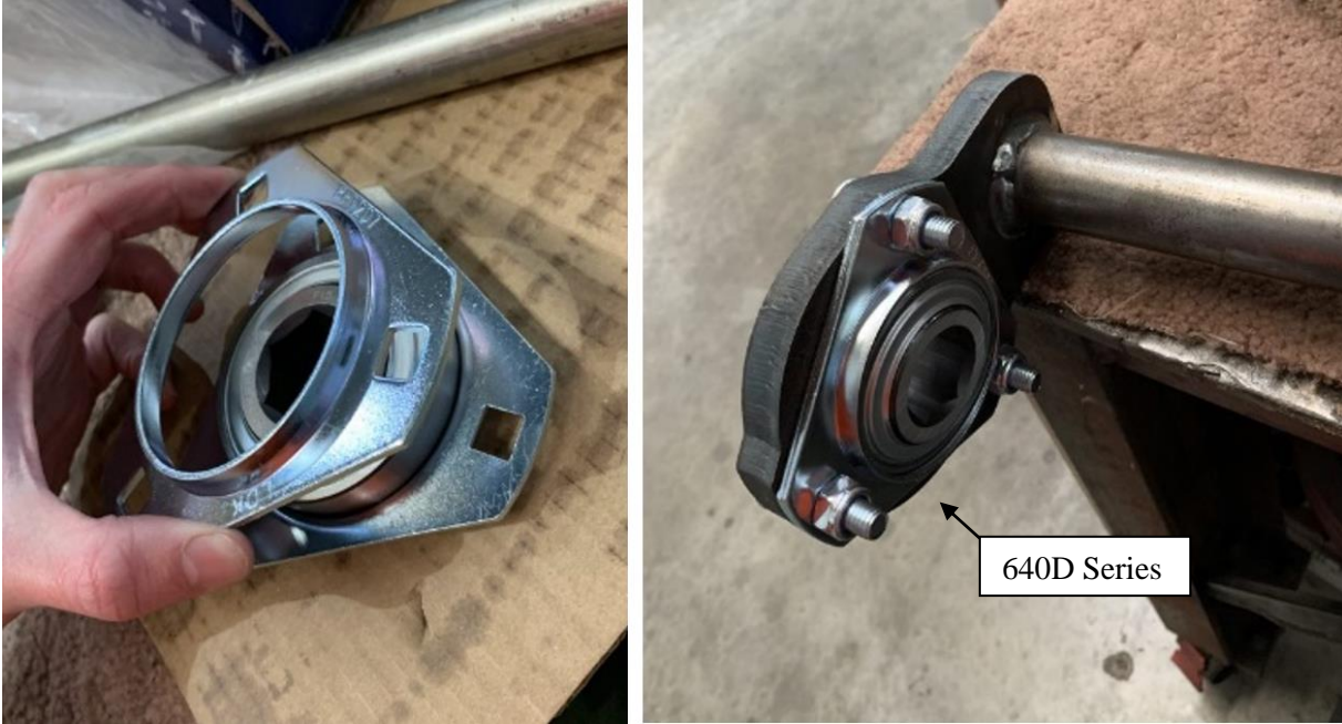
Figure 14: Bearing fitting in bearing housings (left). Bearing housing fitted to drive end of crankshaft (right).
