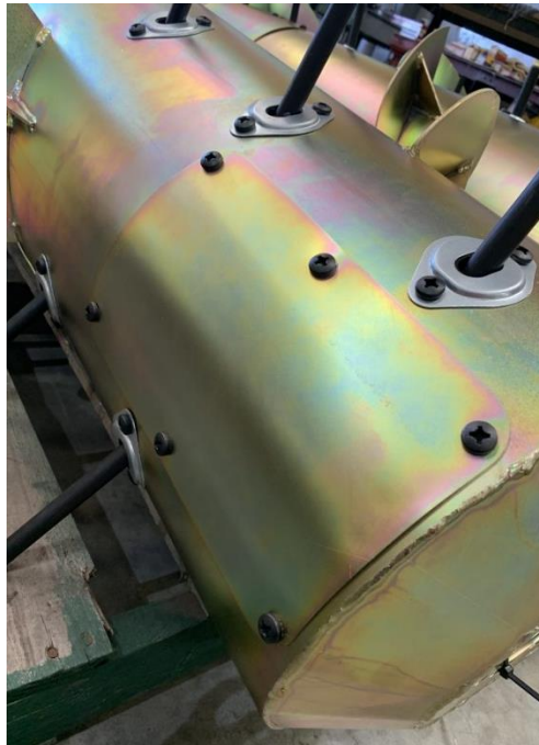
Figure 18: Fitted inspection hatch cover.
