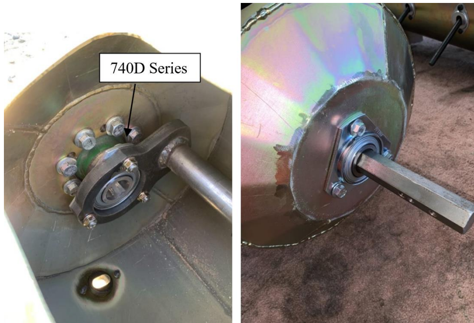
Figure 15: Internal crankshaft orientation (left). Securing the crankshaft at the idle end (right).
