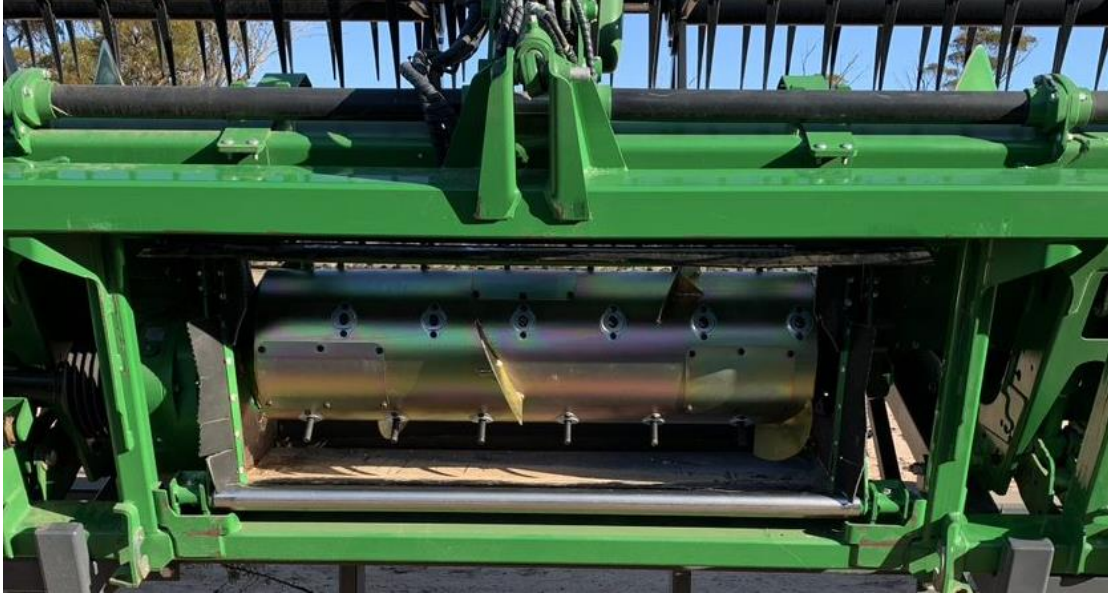
Figure 13: Fully installed new iPaddock Typhoon.
