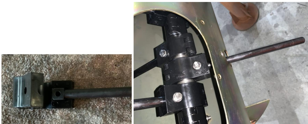
Figure 16: Finger in finger holder (left). Finger holder assembly onto crankshaft (right).
