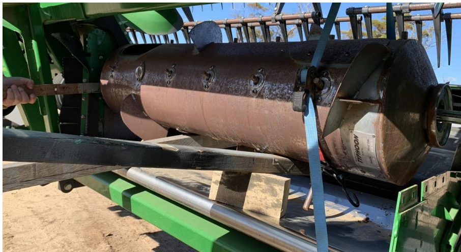
Figure 8: Using wooden beams to lever and maneuver the drum shell.
