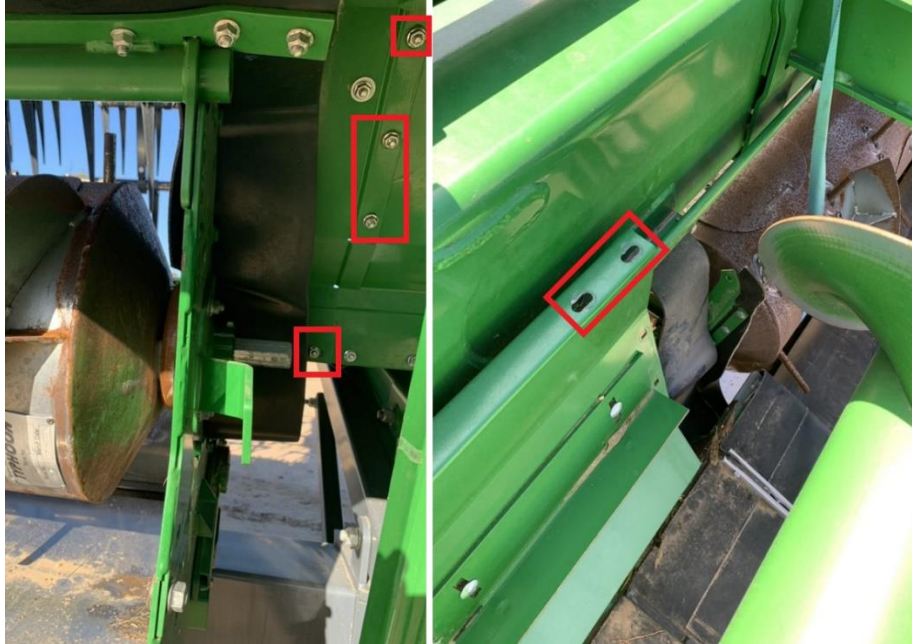
Figure 3: Location of bolts securing bracket (left). Bolts on top of header front (bracket is removed) (right).
