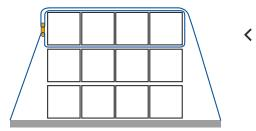
Top layers can be securely belly wrapped to stop the center of load shifting forward under braking. There is no need to pyramid stack, therefore maximizing payloads.
