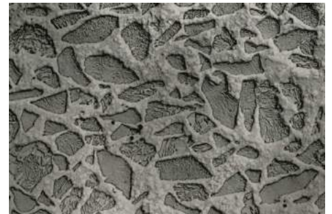
Coating with densely packed hard tungsten carbides in a matrix to form an impenetrable barrier to abrasive particles.
