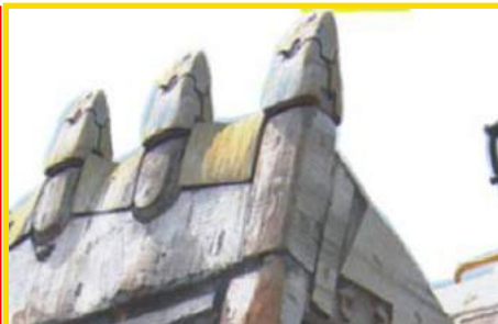
DO 385 Bucket Teeth for Quarry Industry Abrasion + Impact Resistance
