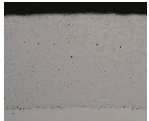
Microstructure of a 2-step sprayed & fused coating
