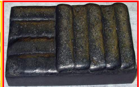
DO 390 can be built up to a of up to 12.5mm (1/2 inch)
