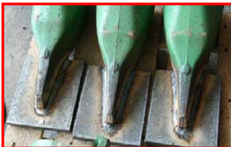
Cutting Teeth for Dredging Industry thickness Abrasion + Impact Resistance
