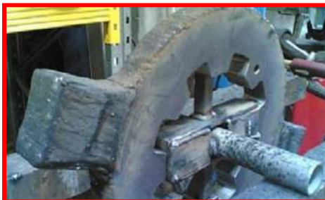
Shredder Hammer for Waste & Recycling Industry. Abrasion + Impact + Heat Resistance
