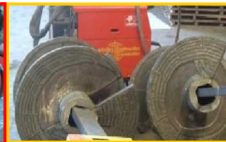
Clay Mixer Screws for Brick & Tile Abrasion + Impact resistance
