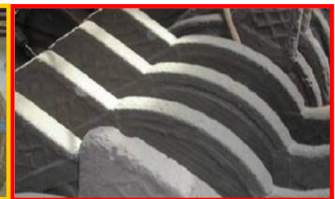
Sinter Crusher Hammers for Steel Ind. Abrasion + Impact resistance
