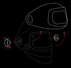
For extended non-welding work, just unscrew the two dials to completely remove the welding visor and re-attach the dials again, reducing the helmet weight by over 35%.
