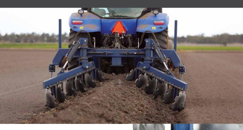
Now available is our heavy duty Disc Banker which is a fast and efficient way to build or renovate irrigation banks.
