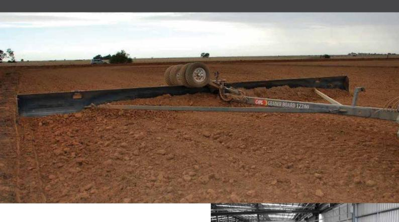
Our robustly designed 35, 40 & 45 foot Grader Boards are designed with a hydraulic fold action for easy transportation.
