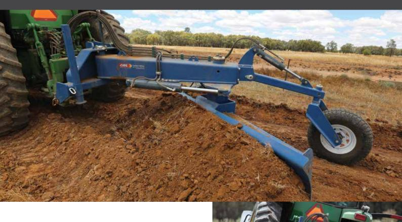
The new Heavy Duty Grader Blade from Collier & Miller features heavy plate construction and large diameter pins to withstand strenuous dirt forming operations, making it ideal for building and repairing roads.
