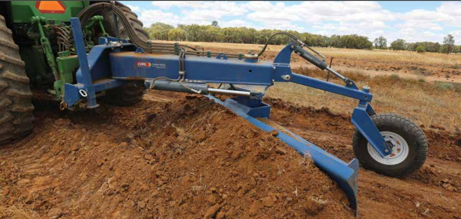
The new Heavy Duty Grader Blade from Collier & Miller features heavy plate construction and large diameter pins to withstand strenuous dirt forming operations, making it ideal for building and repairing roads.
