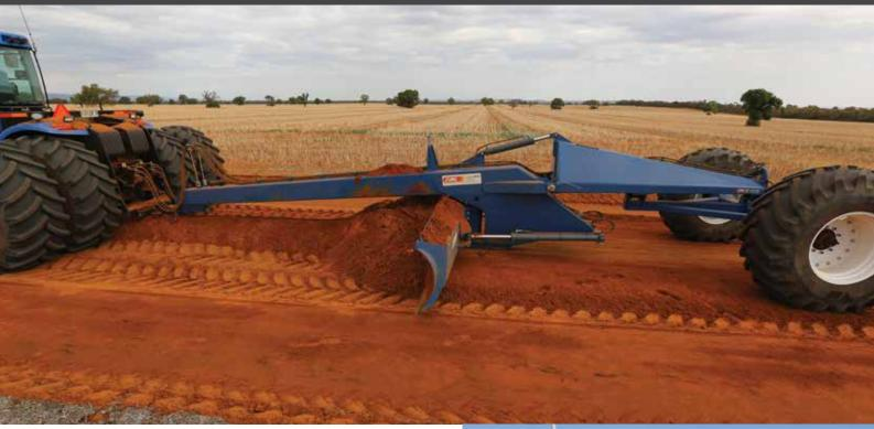
The Collier & Miller Heavy Duty Tow-Behind Grader has been designed to handle the harshest terrain when building or maintaining roads, fire breaks and driveways.
