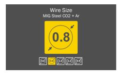
Rotate **SELECT** knob to required wire size then press to select.
