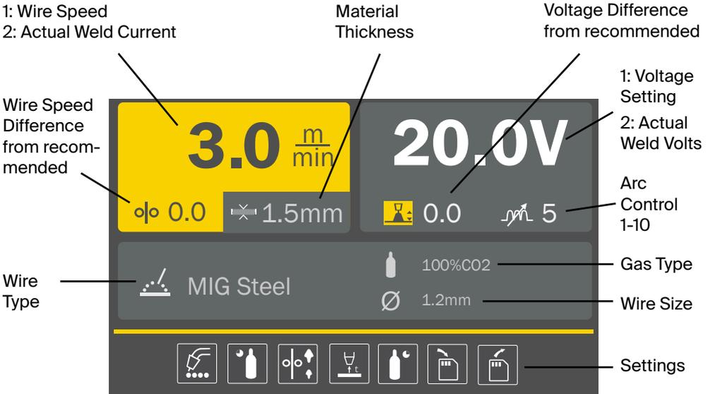
Adjust wire speed by turning the **SELECT** knob.
