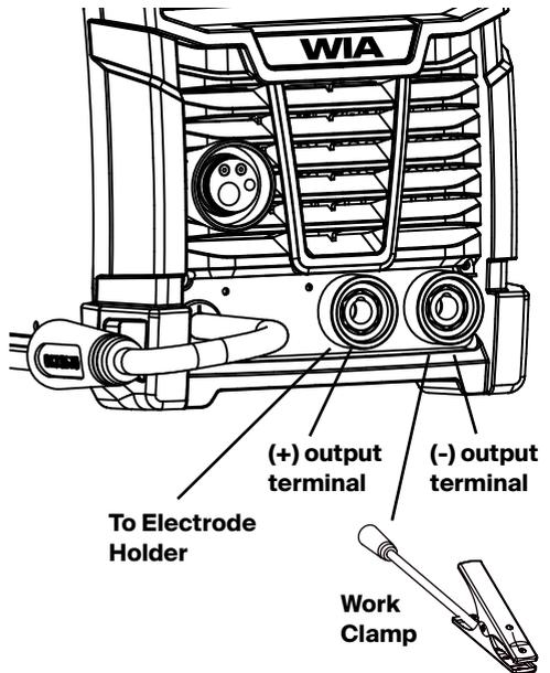
**Fig 6 Connections for stick welding (MMAW), electrode positive**
