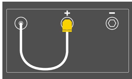
This screen shows information about the correct Polarity connection. Wait for the next screen or press **SELECT**.
