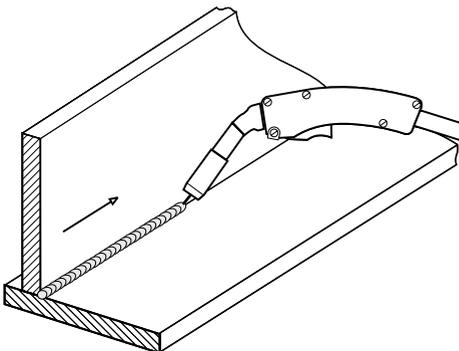
**Fig 5b Gasless Flux Cored Wires**
