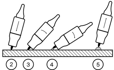
**Fig 8 Lift TIG Operation Procedure**
