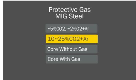
For MIG Steel, rotate **SELECT** knob to required gas option then press to Select.
