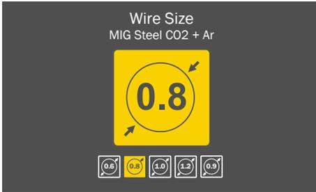
Rotate **SELECT** knob to required wire size then press to select.
