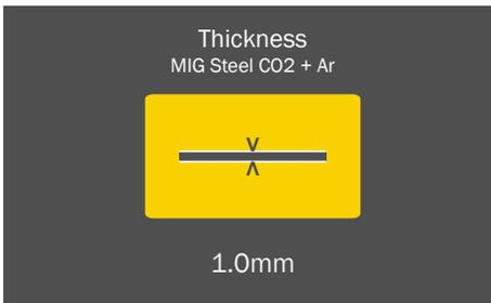
Rotate **SELECT** knob to required material thickness then press to select.
