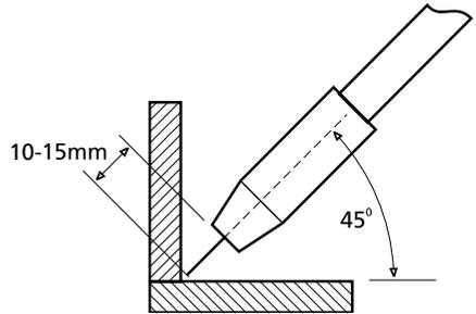
**Fig 5c Wire Stickout for Gasless Welding**
