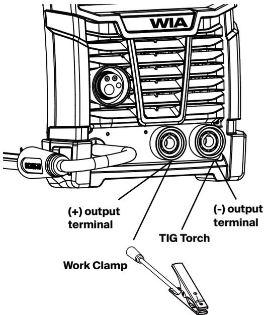
**Fig 7 Cable and hose connections for TIG welding**
