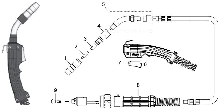
**Fig 15 GUN001 (200 amp) Gun and Cable Assembly**
