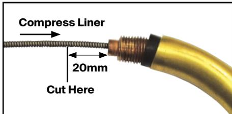
**Fig 16 Replacing the Gun Cable Liner**
