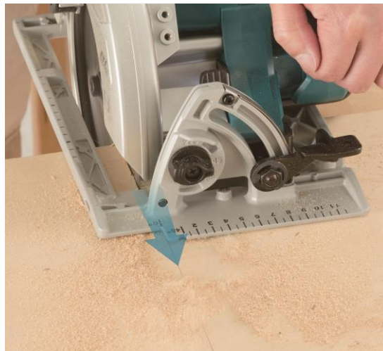
Blower function clears cut line automatically
