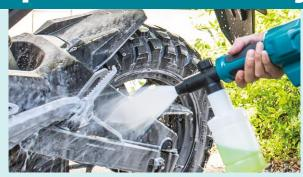
Chemical bottle attaches onto the front of the unit to spray foam over item to be cleaned
