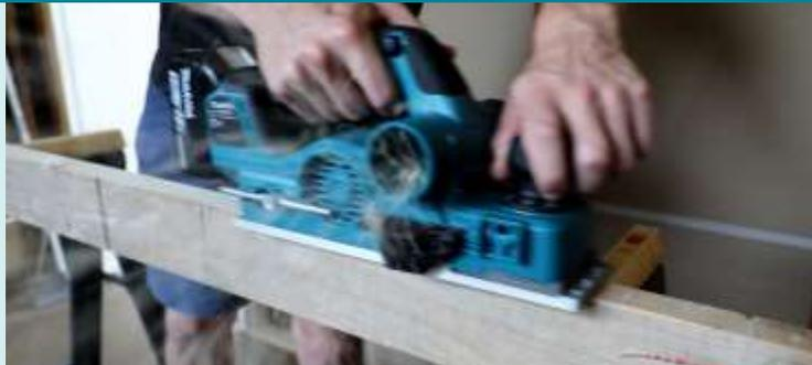
Left & right chip ejection for convenient operation
