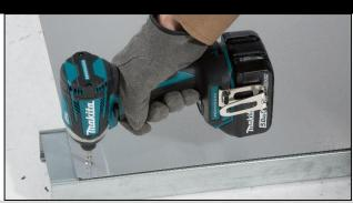
T:Mode: Tightening mode for self drilling screws into metal
