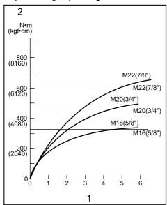
1. Fastening time (second) 2. Fastening torque
