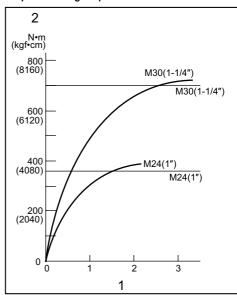
1. Fastening time (second) 2. Fastening torque
