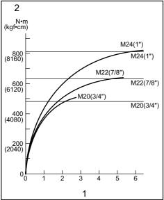
1. Fastening time (second) 2. Fastening torque
