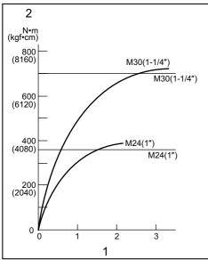
1. Fastening time (second) 2. Fastening torque
