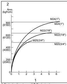
1. Fastening time (second) 2. Fastening torque
