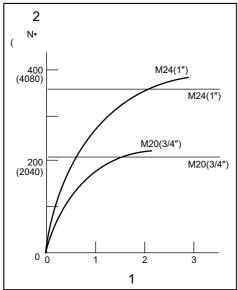
1. Fastening time (second) 2. Fastening torque
