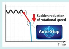
Active feedback sensors shut down the tool in the event of a kickback
