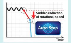
Active feedback sensors shut down the tool in the event of a kickback **Durability**
