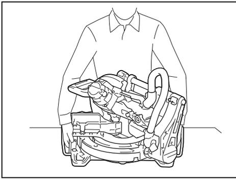
**▲WARNING:** Stopper pin for carriage elevation is for carrying and storage purposes only and not for any cutting operations. The use of the stopper pin for cutting operations may cause unexpected movement of the saw blade resulting in kickback and serious personal injury.
