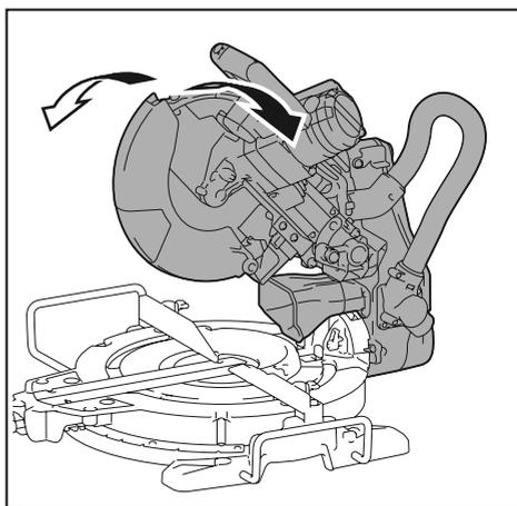
If the pointer does not indicate the 45° position, align it with 45° position by turning the adjusting bolt on the opposite side of the bevel angle scale.
