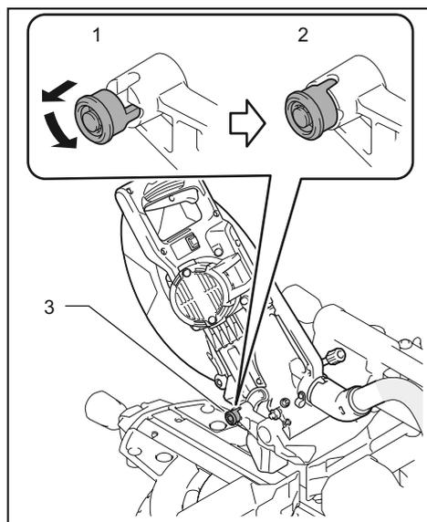
▶ 1. Unlocked position 2. Locked position 3. Stopper pin
