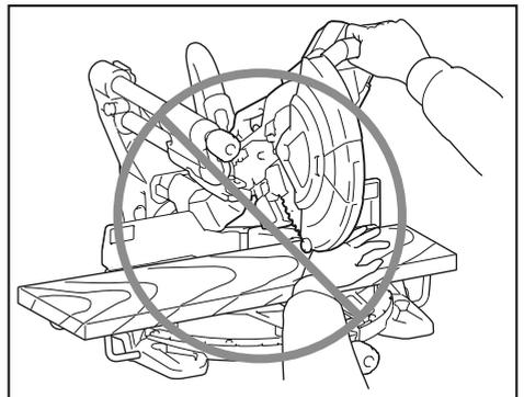
6. **Do not reach behind the fence with either hand closer than 100 mm from either side of the saw blade, to remove wood scraps, or for any other reason while the blade is spinning.** The proximity of the spinning saw blade to your hand may not be obvious and you may be seriously injured.
