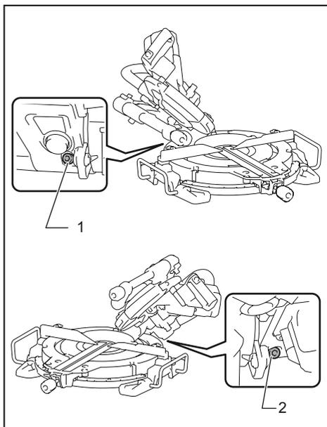
► 1. Left 45° adjusting bolt 2. Right 45° adjusting bolt
