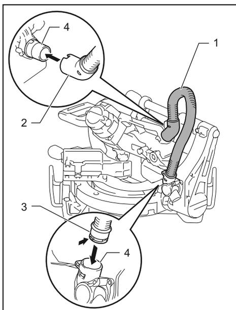
► 1. Dust extraction hose 2. Elbow 3. Sleeve 4. Port
