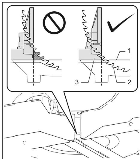
► 1. Top surface of turn base 2. Periphery of blade
