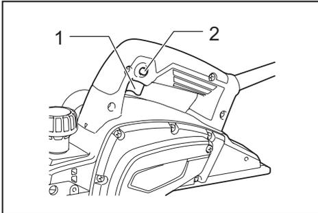
► 1. Switch trigger 2. Lock button or Lock-off button
