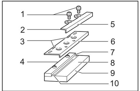
► 1. Screws 2. Adjusting plate 3. Planer blade locating lugs 4. Gauge plate 5. Heel of adjusting plate 6. Set plate 7. Inside flank of gauge plate 8. Gauge base 9. Back side of gauge base 10. Mini planer blade
