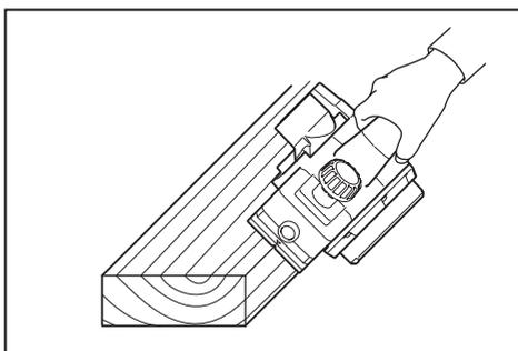
To make a chamfering cut as shown in the figure, align the "V" groove in the front base with the edge of the workpiece and plane it.
