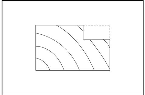
To make a stepped cut as shown in the figure, use the edge fence (guide rule).
