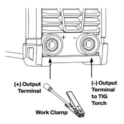
Fig 4 Cable Connections for TIG welding
