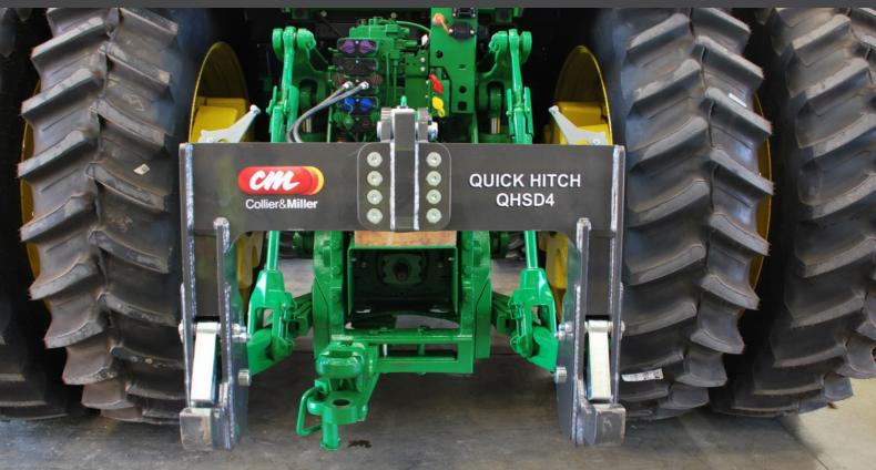
Collier & Miller Quick Hitches are designed and manufactured in NSW, Australia to enhance onfarm productivity when switching three-point linkage implements. Our premium hitches provide a secure, dependable, and efficient solution for changing over linkage-mounted attachments.
