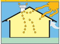
Under eave vents aid roof space air circulation. Install two per Spinaway. Spinaway turbo ventilators exhaust the very hot air that becomes trapped in the space between the ceiling and roof covering. This prevents heat radiation into rooms and helps lower inside temperatures.
