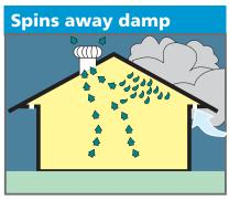
Under eave vents aid roof space air circulation. Install two per Spinaway.
