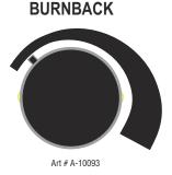
Burnback time is used to adjust the amount of MIG wire protruding from the MIG torch contact tip (stick out) after the completion of welding. Rotating the Burnback control in a clockwise direction increases the Burnback time. Rotating the Burnback control in an anticlockwise direction reduces the Burnback time.
