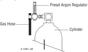
Figure 4-4 Fit Regulator to Cylinder
