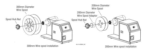
Figure 5-2 WeldSkill 250 & 350 WF Setup and WF Spool Hub
