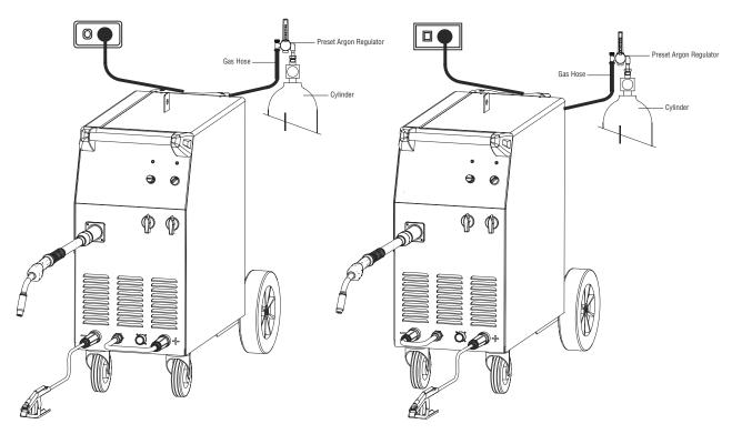
Setup for MIG (GMAW) Welding with Gas Shielded Shielded MIG Wire
