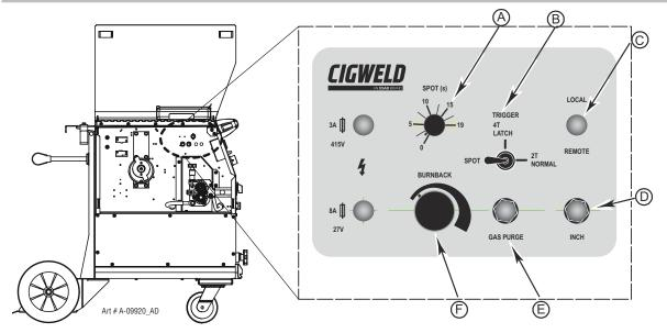
Figure 4-3 Internal welding controls
