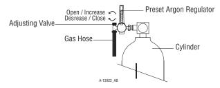
Figure 4-5 Adjust Flow Rate
