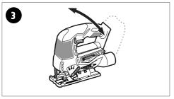
Rotate the base plate to the desired angle (0, 15, 30, 45°). Push the base plate towards the front of the unit ensuring the teeth are either side of the locking tab.
