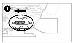
1. Push switch towards the front of the unit to put into extraction mode. This will eject the dust out the dust extraction port (3)
