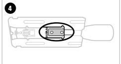
4. Re-tighten the 2 bolts with the hex key, ensuring the base plate is securely positioned at the correct angle.
