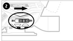
Push switch towards the rear of the unit to put into blower mode. This will blow air towards the cutting blade, removing excess debris and increasing visibility.
