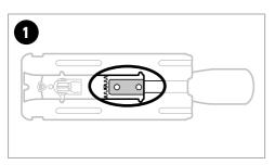
1. Use the supplied Hex Key (3mm) to loosen the 2 bolts on the underside of the Jigsaw.
