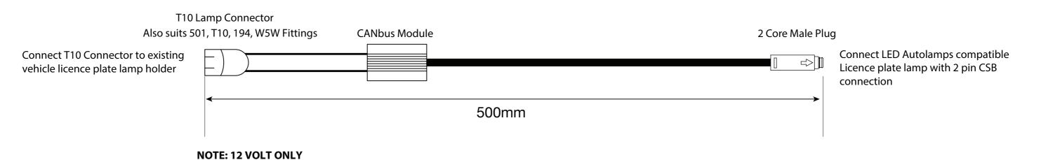
**NOTE:** CANbus Module can generate heat with temperatures ranging up to 95°C. Please keep away from any plastics or anything that could melt. Best to be mounted to flat metal surface with double side tape.
