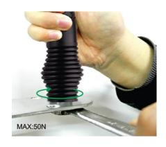
2. Install the fiberglass whip to the elevated feed by turning in a clockwise direction and hand tighten only MAX. 15N.
