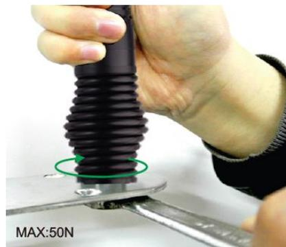
3. Remove the cap from the top of the spring base and install the fiberglass extension pole on to the base by turning in a clockwise direction and secure in place with the grub screw (using the hex key provided). Hand tighten only MAX. 15N.
