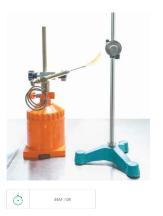
Dynamometer Test To measure the load when the product is reopened.
