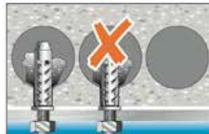
Incorrect installation - not recommended
